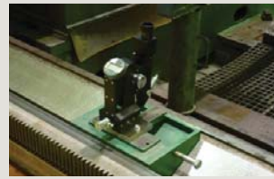
Guideway condition analysis
