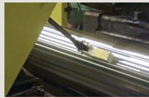
Eddy current & ultrasonic inspection system integrated with Sinumerik 840D CNC
