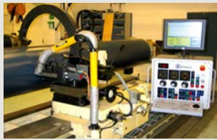
3D TurnControl™ • High precision turning system for supercalender lathes
