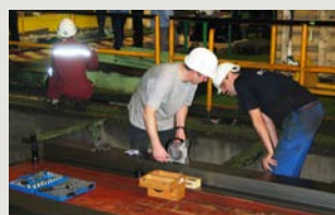
Mechanical refurbishing • rescraping • alignment
