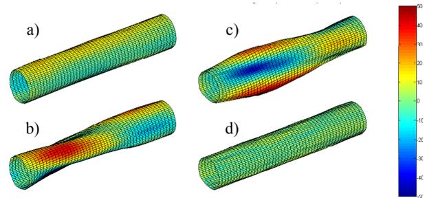
**Fig. 4.** Geometry of the test roll with traditional grinding at a low speed of 50 m/min (a) and at a production speed of 1120 m/min (b), and after predictive 3D grinding at low speed (c) and at production speed (d) respectively.
