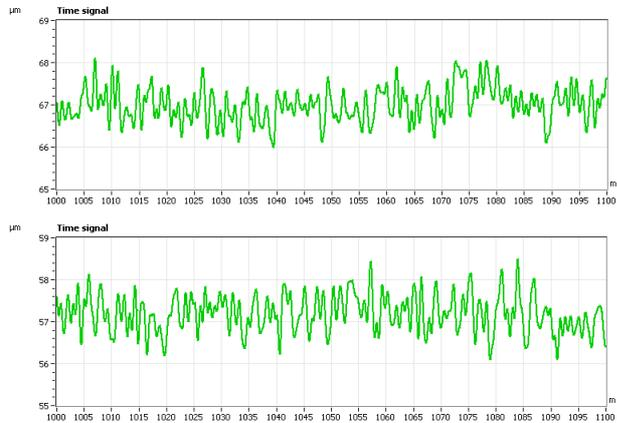
**Fig. 9.** Thickness variation of the coated paper in MD before (above) and after predictive 3D machining.
