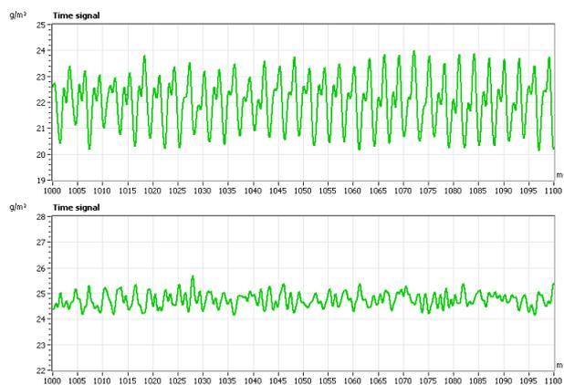
**Fig. 6.** Ash variation of the coated paper in the time domain in MD before (above) and after predictive 3D machining.
