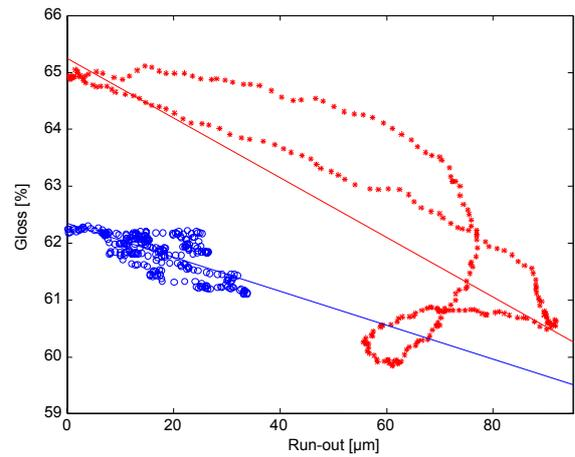
**Fig. 11.** The correlation between the gloss and run-out of the backing roll before (stars) and after (circles) predictive 3D machining.
