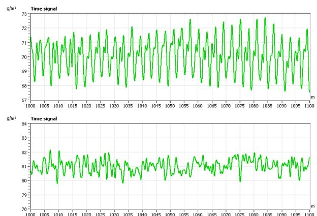
**Fig. 8.** Basis weight variation in the time domain of the coated paper in MD before (above) and after predictive 3D machining.
