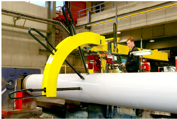
Fig. 3. 3D grinding system provides the desired geometry to within an accuracy of one micrometer [17].
